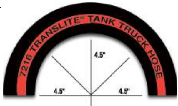
The minimum bend radius is measured to the inside of the curvature.
